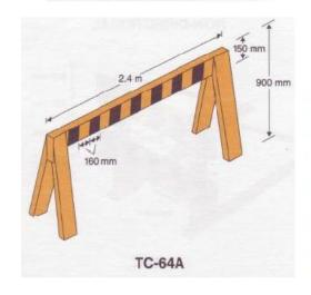
Barricades are used only to protect workers, and MUST NOT be used as delineators to channel traffic. They must not be placed in the Buffer Area of a Temporary Work Zone.
